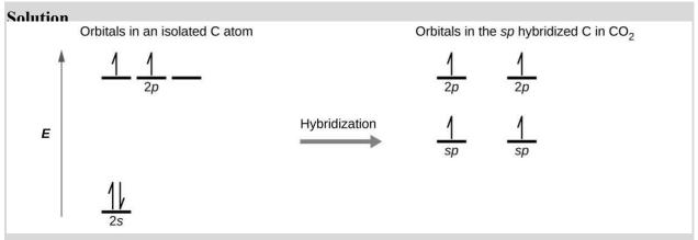
Each of the four electrons is in a senarate orbital and overlans with an electron on an oxvgen atom.
