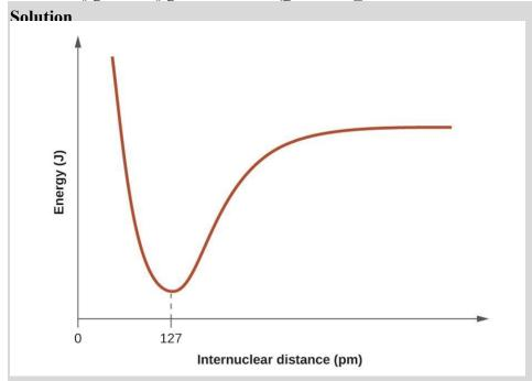
When H and Cl are senarate (the x axis) the energy is at a particular value. As they approach, it decreases to a minimum at 127 nm (the bond distance), and then it increases sharply as you get closer.
